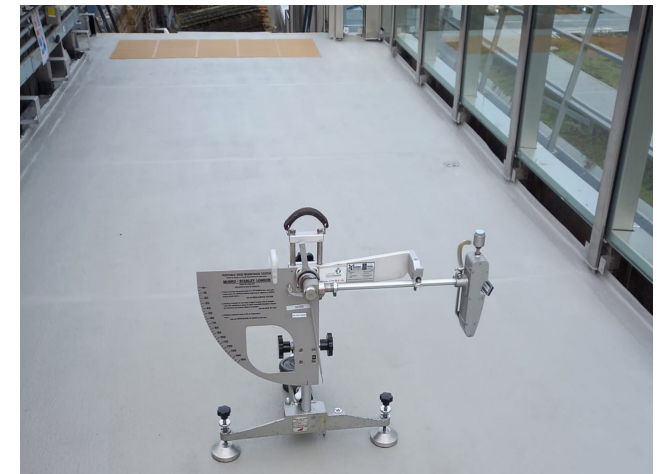
After: Pendulum Test In Progress
